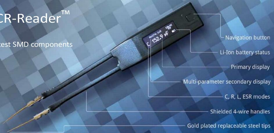
LCR-Reader™ is a professional quality, low cost LCR and ESR-meter. It provides the perfect solution for testing and identifying Surface Mount Devices (SMD), as well as troubleshooting complex electronic systems.
